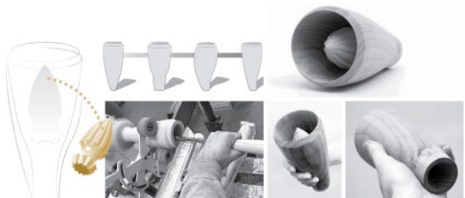
Figure 16. Citrus Juicer 2012. Shane Zeigler. 4-Axis CNC milling (interior reamer) and hand-guided turning (vessel).
