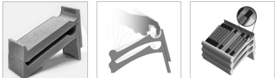
Figure 5. Tool Cradle Project 2012. Alex Chiles. Left: Foam Form Study; Middle: Ergonomic Study; Right: CAD Model
